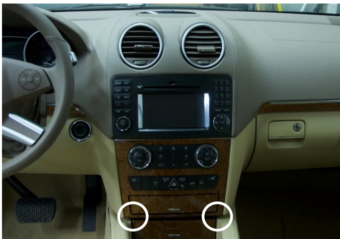
1) Pull out on bottom of HVAC panel
